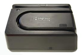
Incorporating E13b and CMC7 formats coupled with an incredibly reliable MSR (badge reader) as well as an optional Smart Card reader, Chequemate 250 is the ideal device for your teller front end needs.
